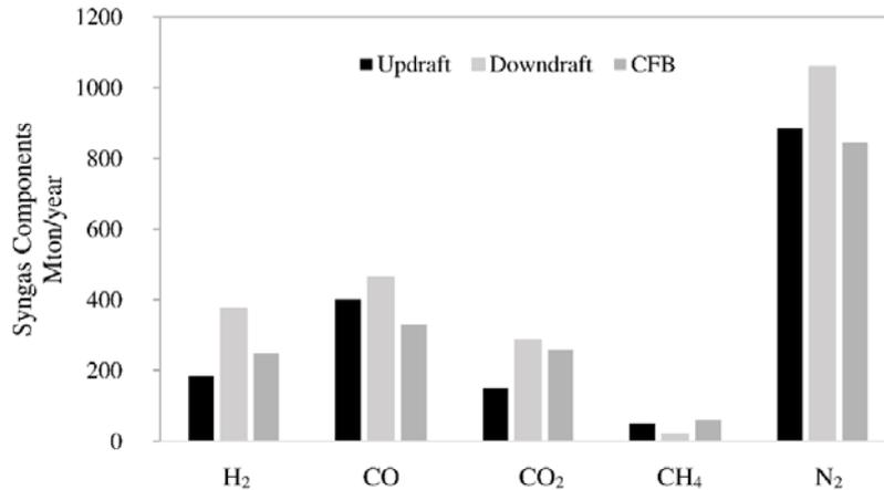
**Fig.2.** Production rate of different syngas components from updraft, downdraft and CFB systems
