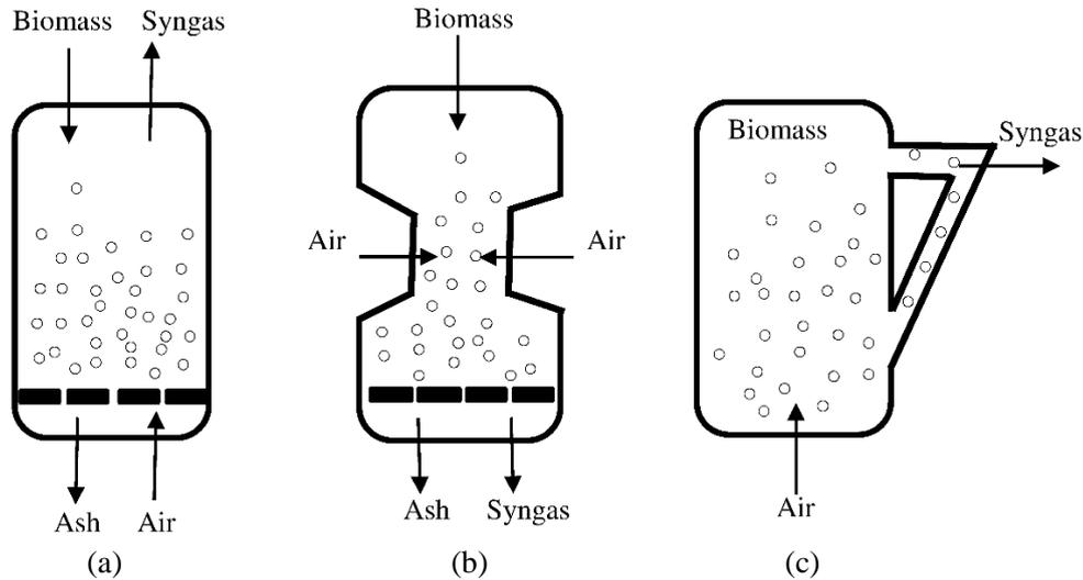
**Fig.1.** Different gasification technologies (a) updraft, (b) downdraft, (c) circulating fluidized bed (CFB)
