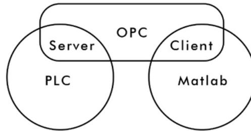
**Fig. 4.** Matlab, PLC and OPC connection structure
