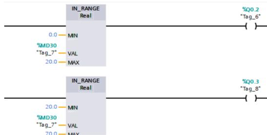
Fig. 8. Activated physical output
