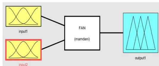
Fig. 10. (input1=temperature, input2=humidity, output=speed)
