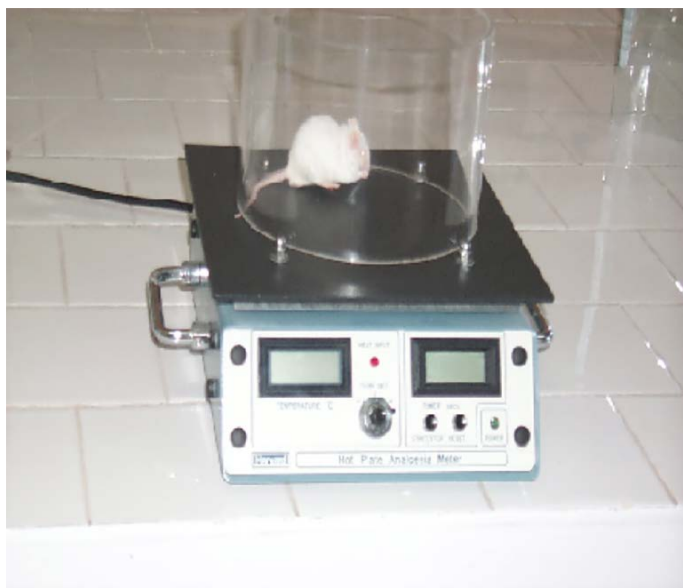
Figure 1. A harvard hot plate analgesia meter (Edenbridge, England) [10].
