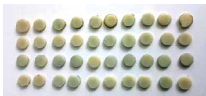
Figure 2. The provisional restorative materials evaluated in terms of colour change have been presented below from top to bottom: listerine, colgate, sensodyn and green tea samples, respectively.
