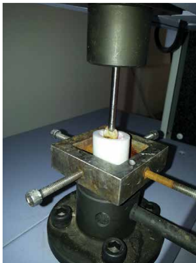
Figure 4. Sample attached to the Universal Testing Machine for fracture test.
