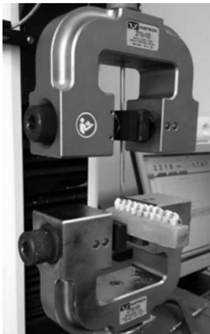
Figure 2. Test apparatus used for shear bond strength testing.
