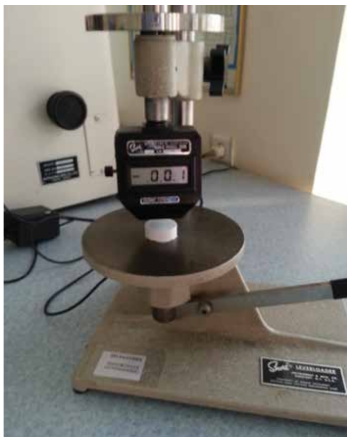
Figure 2. Shore A testing of the specimens.
