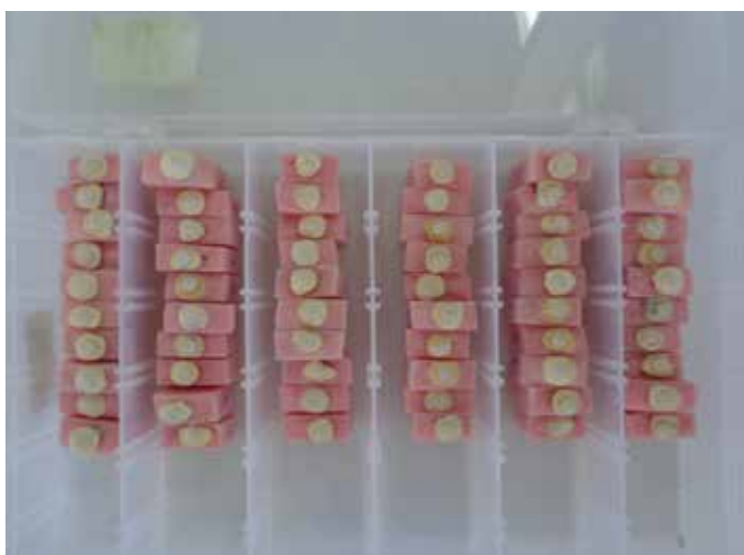
Figure 1. All specimens prepared and embedded in autopolymerizing acrylic resin.
