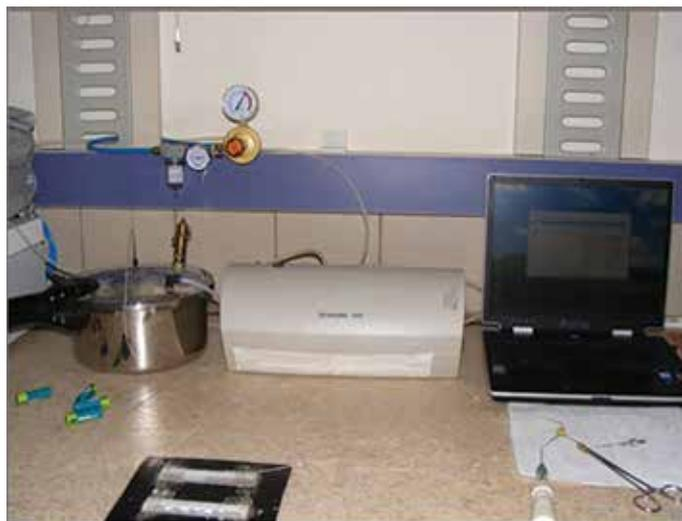
**Figure 1.** Fluid flowmeter used for microleakage measurements.
