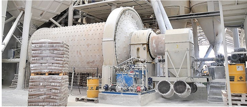
Figure 2. Image of calcite grinding mill (Classic ball mill)
