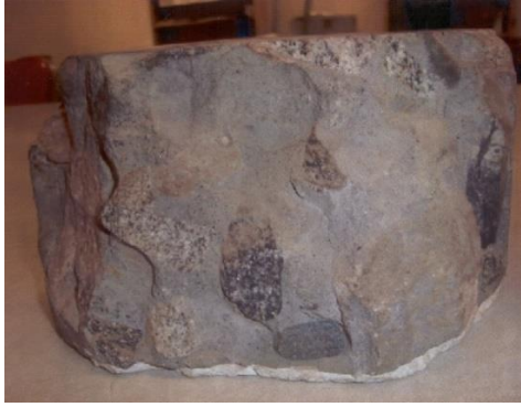
Fig. 2. A sample of PAC prepared by the conventional method for the restoration of Barker Dam
