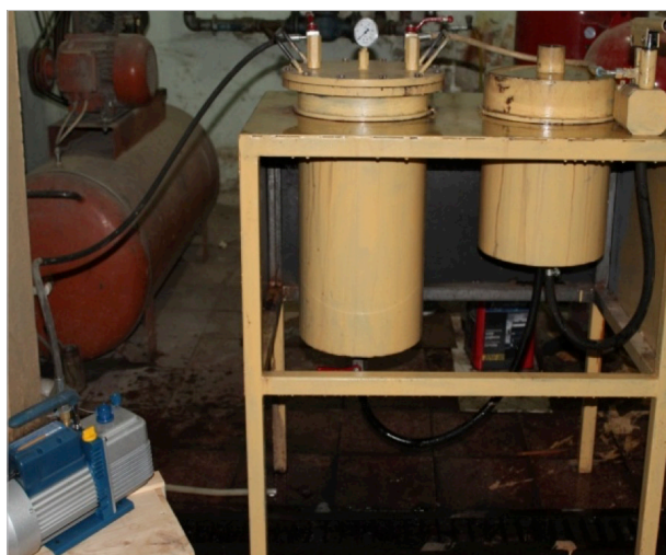
Figure 2. Impregnating device employed in the impregnation process
