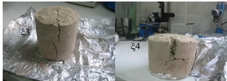
Figure 3. Deformed samples after freezing-thawing ( \xi_3 and \xi_4 )
