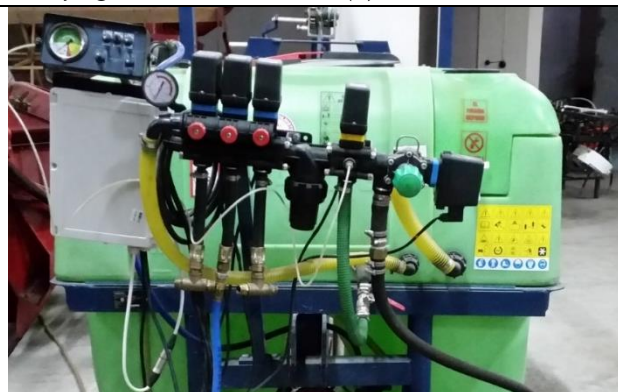
Figure 2. Sprayer and electro-valve installation
