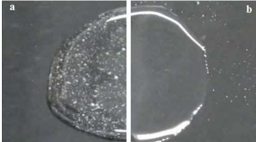
Figure 4. (a) Matrix resin with air bubbles and (b) matrix resin with air bubbles removed
