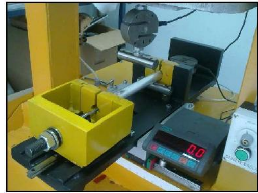
Figure 3. Test on three point bending machine with pre-stress device
