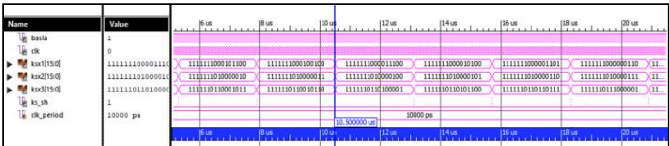
Figure 11. Simulation results of Xilinx ISE 14.7 of DP-based 8I-8Q fixed-point number standard SEA oscillator
