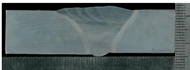
Figure 7. Macro photo of welded sample with GTAW
