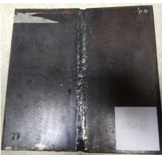
Figure 5. Welded plates with SMAW and GTAW
