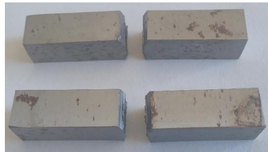
Figure 14. Test specimens after impact tests
