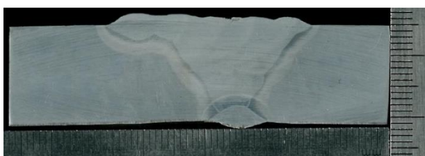
Figure 6. Macro photo of welded sample with SMAW
