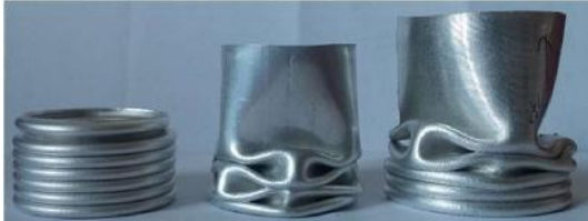
Figure 5. Axisymmetric, diamond and mixed deformation modes of tubes (respectively from left)
