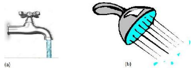
Figure 1. (a) Regular FDM single carrier, all water comes from the single big faucet (b) OFDM, the same amount of water comes from different holes [5]
