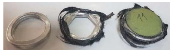
Figure 13. Changes in deformation modes with different reinforcement materials
