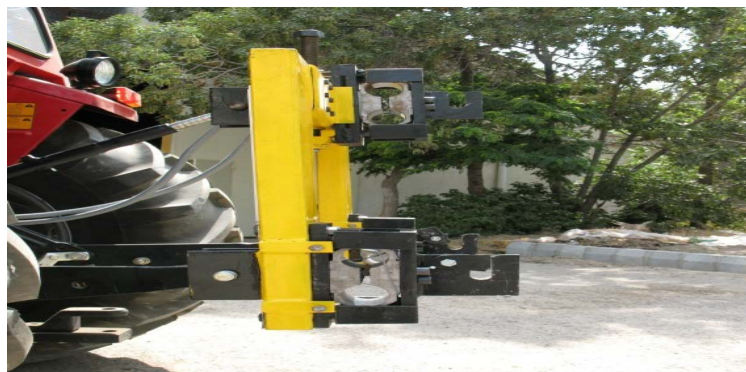
Figure 2. Three-point hitch dynamometer was used to measure draught and vertical force.
