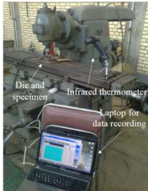
Figure 3. Thermometer installed on the table of angle grinder for measuring instantaneous temperature.
