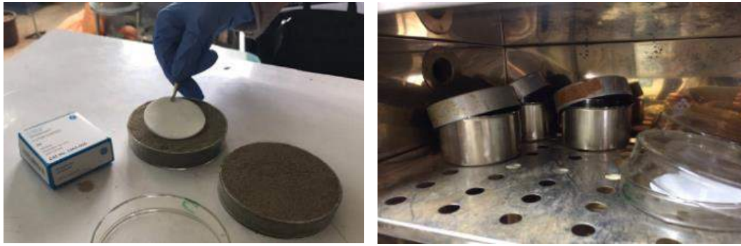
Figure 2. Sampling: a) Removing middle filter paper by using tweezers b) Samples left inside oven overnight
