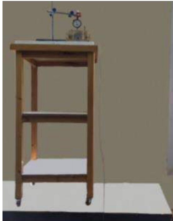
Figure 4. Hanging column test apparatus
