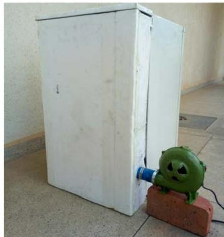
**Fig. 1.** The refrigerator fitted with the drying closet
