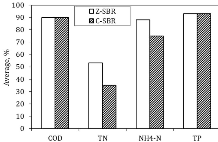
Fig. 1. Pollutant removal performance of C-SBR and Z-SBR.
