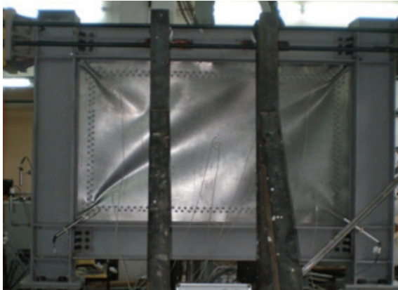
Figure 11 - Specimen TL infill plate at 1\delta_y displacement mode shape
