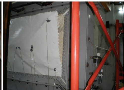
Figure 22 - SP1 Specimen, Plate was torn and completely separated from panel at 9\delta_y
