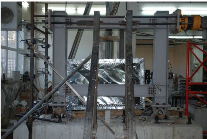
Figure 34 - When the plate yields, removing infill plates from the connecting structural elements can be easily performed
