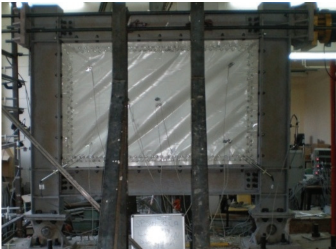
Figure 25 - Overview of the specimen at the -7\delta_y (42.00 mm) displacement step.
