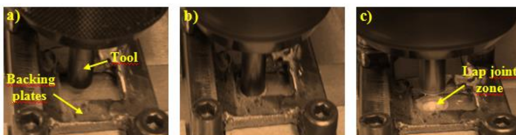
Figure 4. FSSW process: a) rotating tool prior to penetration into the lap joint; b) tool shoulder makes contact with the part, making heat and the joint zone; c) retraction of the tool from the lap joint zone.
