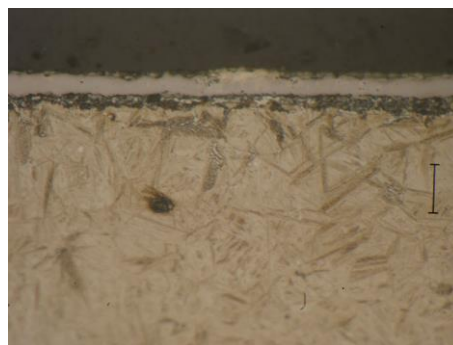
Figure 5. Optical micrograph showing the surface of the interstitial-free steel first titanium diffused at 1000 °C for 2 hours and then boronized at 900 °C for 45 min by applying a current density of 0.10 A/cm 2 (Scale length: 10 µm)
