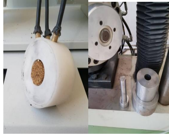
Figure 2. The final shape of sample and mould
