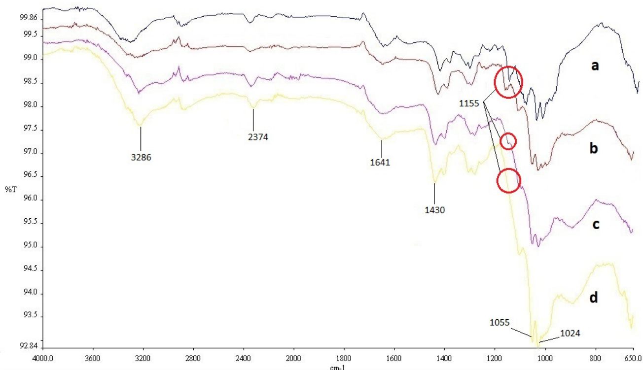
Figure 4. FTIR analyses of fabric samples: (a) unaged, (b) 250 hours treated, (c) 500 hours treated, (d) 750 hours treated
