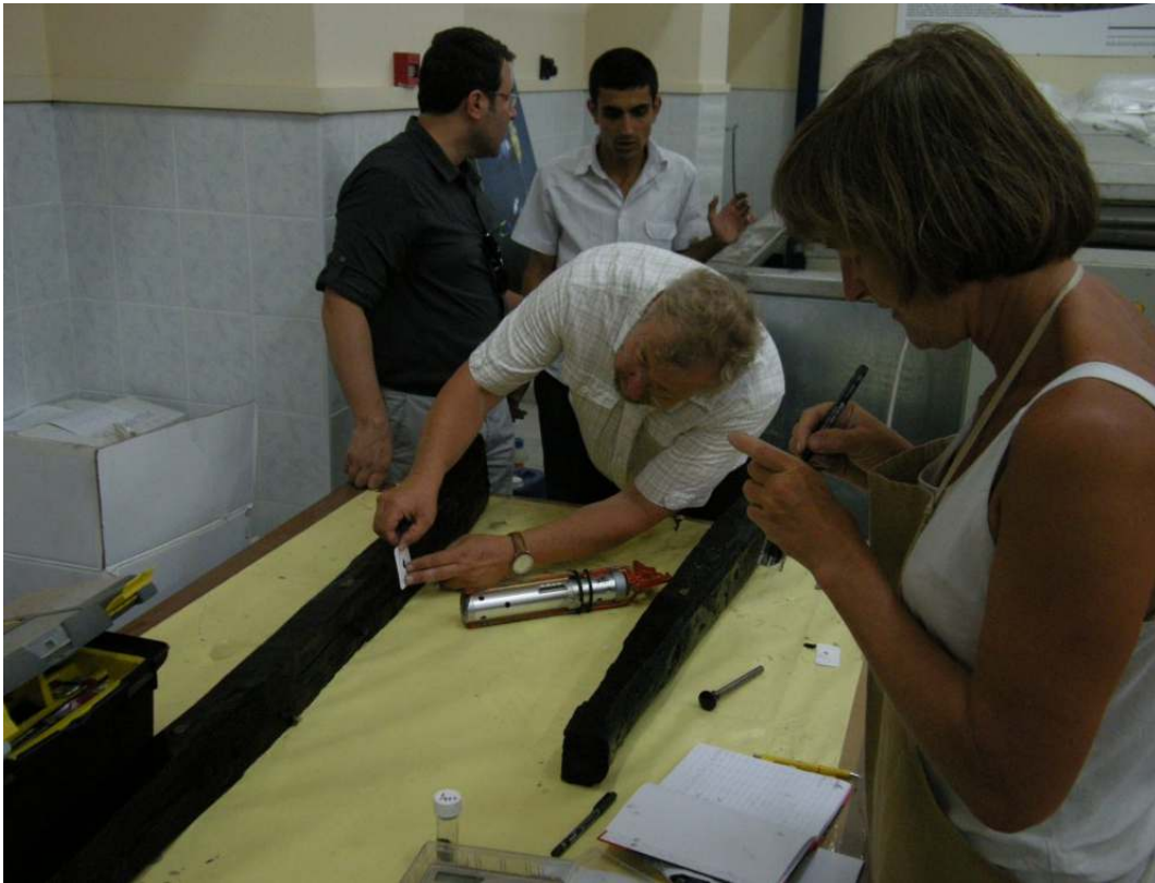
Fig. 2 The process of taking samples from the woods to identify the maximum water content.
