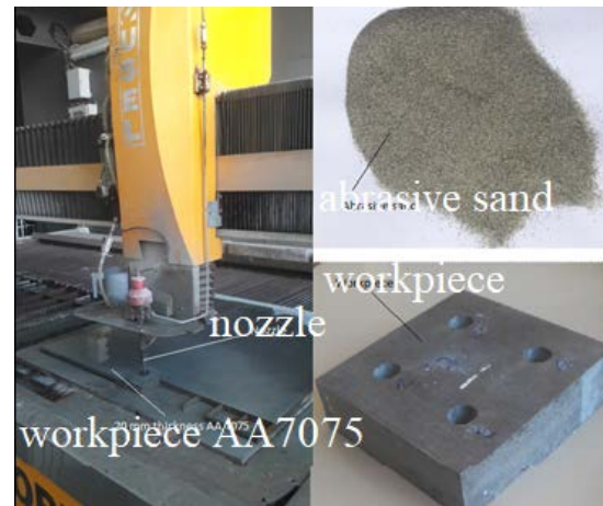
Figure 1. USEL INTERJET CNC WJ 2040 machine, abrasive sand and workpiece
