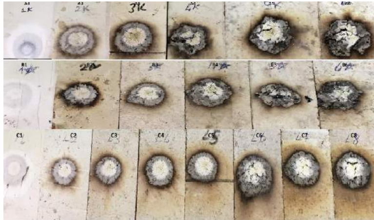
Figure 4. Combustion behavior of test boards for total of 300 seconds.
