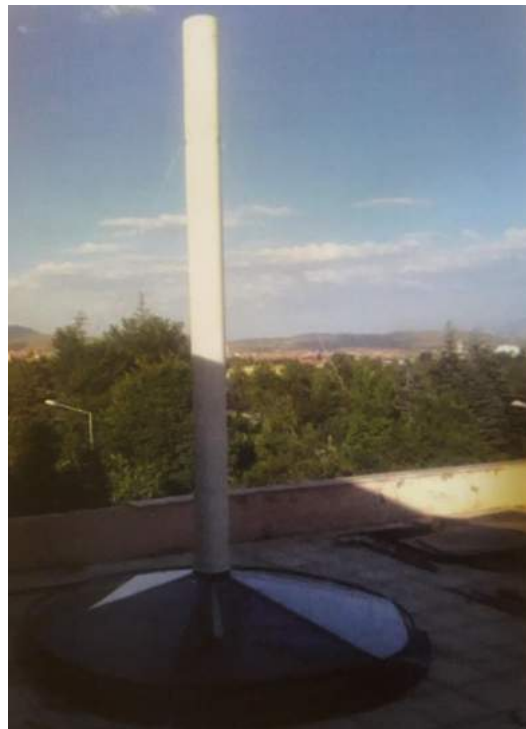
Figure 2. Assembly of the solar chimney
