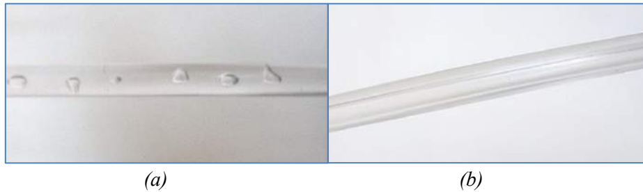
Figure 6. PS rod optic cable samples (a), and hollow rod samples (b)
