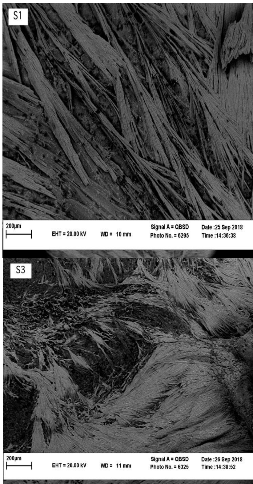
Figure 6A: SEM pictures of lead adsorption (200 times magnified) of starch (0.2 g) chitosan (S1), starch (0.2 g) chitosan- graft -pectin (5 g) (S3).
