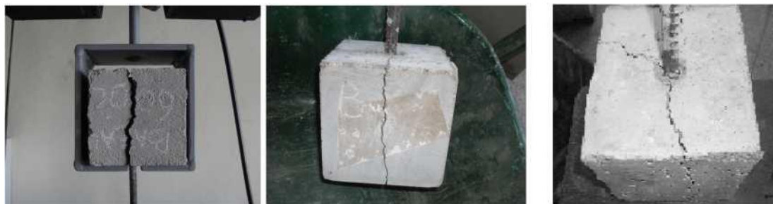
Figure 6. Failures in the samples after the Pull-Out Test.
