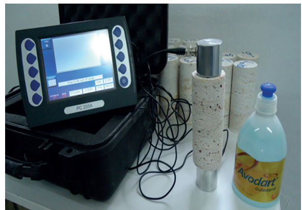
Figure 1. Sound velocity test equipment
