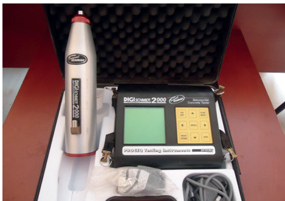
Figure 2. Schmidt hammer hardness test equipment
