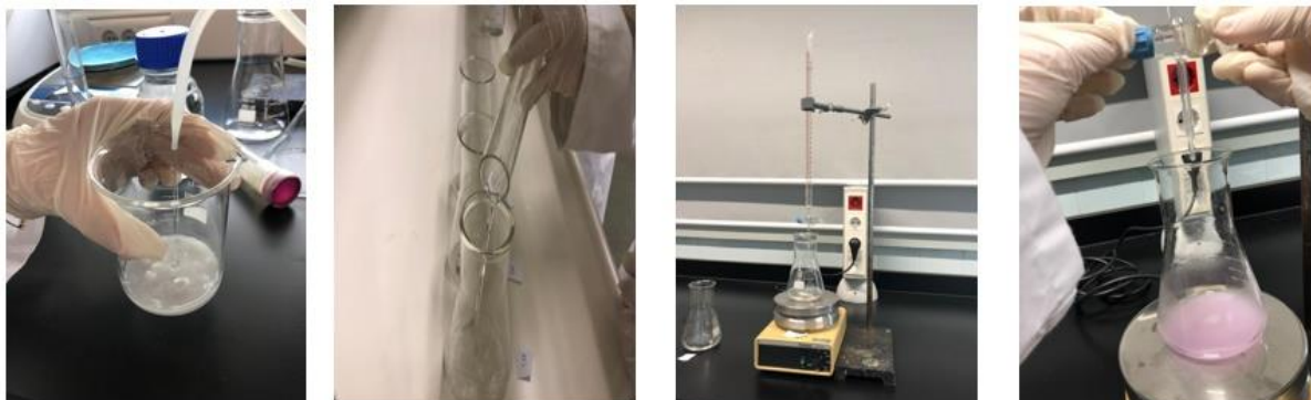
Figure 4. Determination of the acidity index of biodiesel
