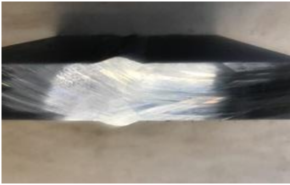
Pic.1. Welded part with X groove
