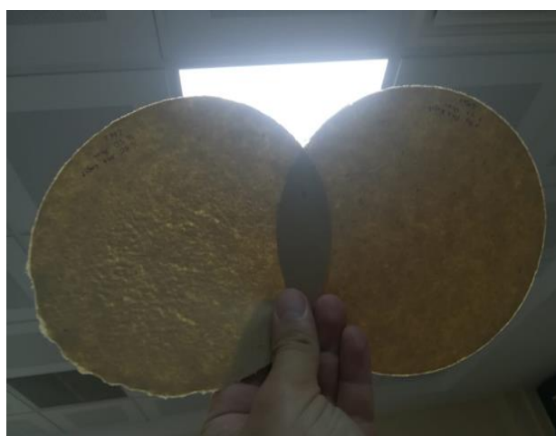
Figure 3. Paper obtained from 50% rose pulp 50% waste paper on left. Paper obtained from 30% rose pulp 70% waste paper on right
