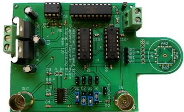
Fig. 11. Constructed system board PCB.
