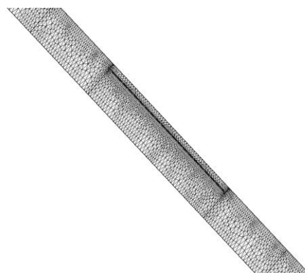
Fig 1. Reactor model, showing the mesh, used in the simulations (1/8 of the whole model). The gas inlet is from the left. The mini monolith is 1 cm long and has a 21 μm catalyst layer on all walls
