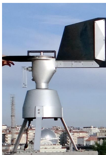
Figure 1. Hirst-type pollen and spore trap (Lanzoni VPSS 2000)
