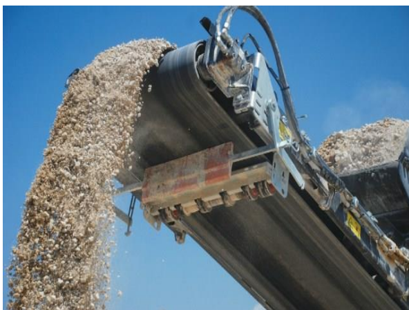
Figure 5. Concrete waste recycling [22]
