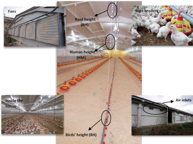
Figure 3- Measurements levels and general views of the broiler house
