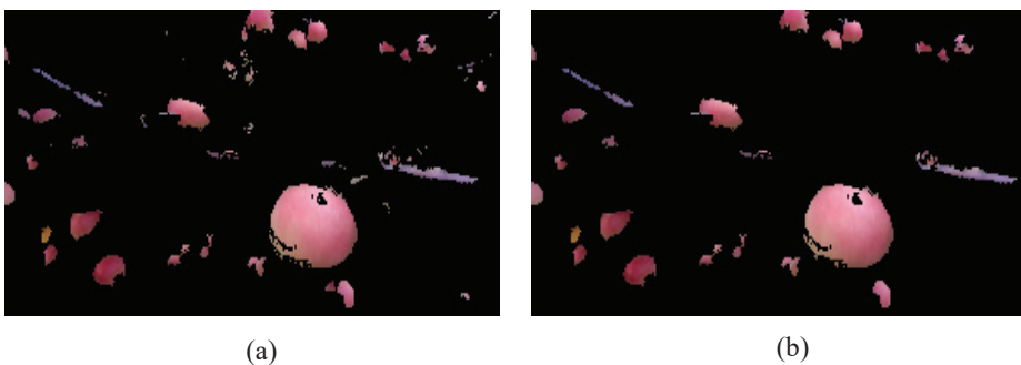
Figure 9- Result of applying morphologic operators over a sample frame that was partially segmented by other segmentation methods. (a), original image; (b), result frame after using morphologic operators
