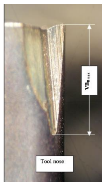
Figure 2. Tool flank wear ( V_c=200 m/min, f_1=0.1 mm/rev, r_3=1.2 mm)
