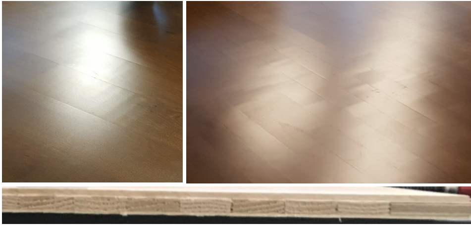
Figure 1: Above: Ondulation at finished multi-layered (laminated) parquet surfaces Below: Tangential stick array in parquet
