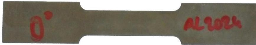
Figure 1. Al 2024-T3 Alloy Tensile Test Specimen.
