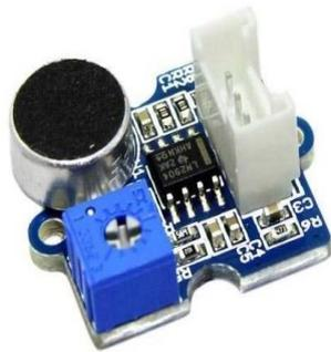
Figure 1. Grove sound sensor and cable connection table
