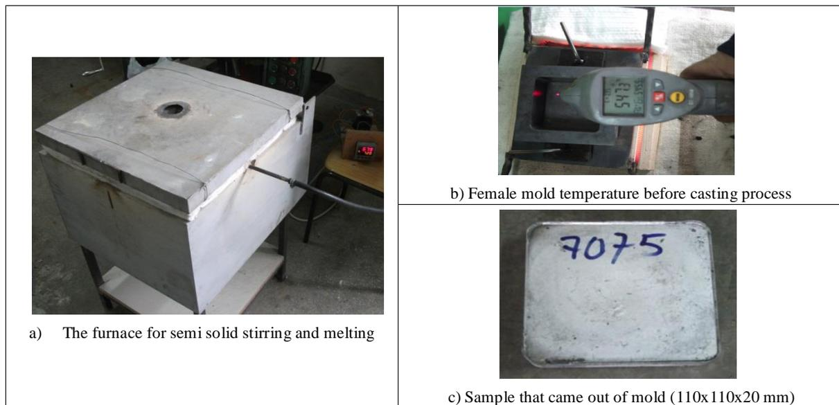
**Figure 1. Experiment details from the AA7075/B<sub>4</sub>C composite production process**
