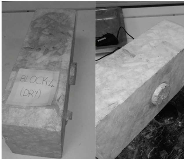
Figure 4 - A sample view from sliding failure of concrete core
