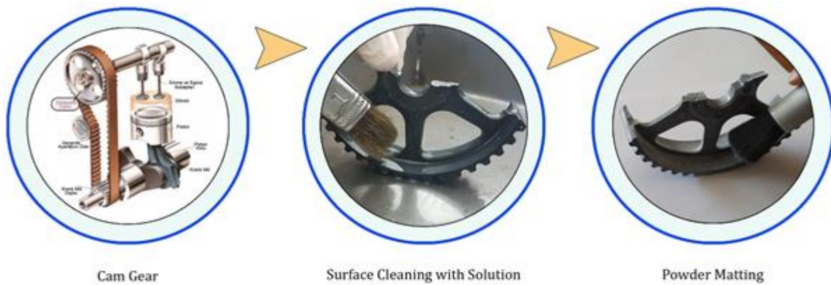
Figure 2. Schematic representation and preparation of the cam gear for 3D scanning
