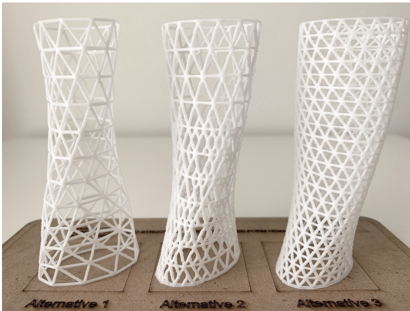
Figure 33 : Three-dimensional fabricated diagrids in 1:2000 scale.
