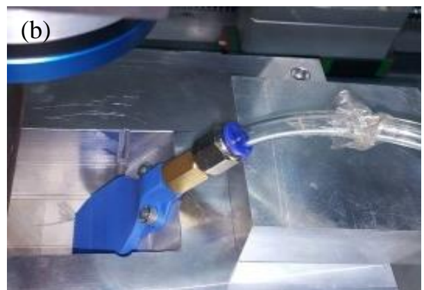
Fig.6. a) Use of weight on both sides of the specimen b) Gas feeding mechanism used for test
