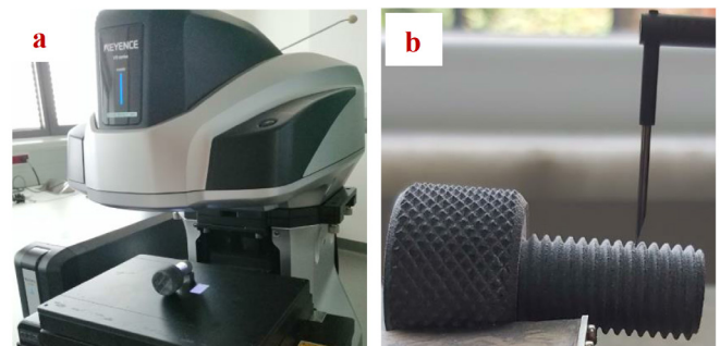
Figure 2. Optical (a) and tactile (b) measurement of the samples.
