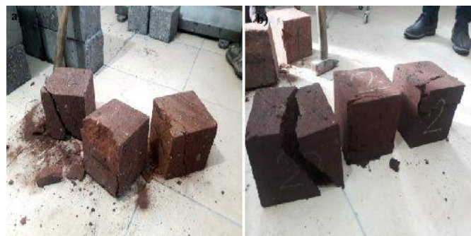
Fig. 5. Ahlat Stone Samples Broken After (a) Air Curing and (b) Water Curing
