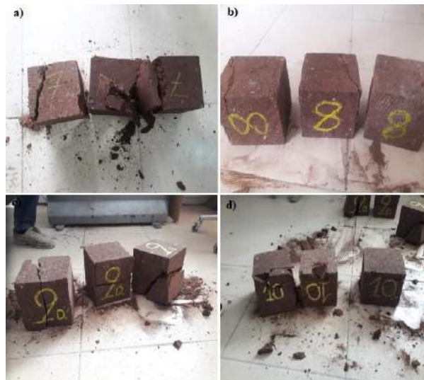
Fig. 7. Ahlat Stone Samples Broken after Combined Curing
