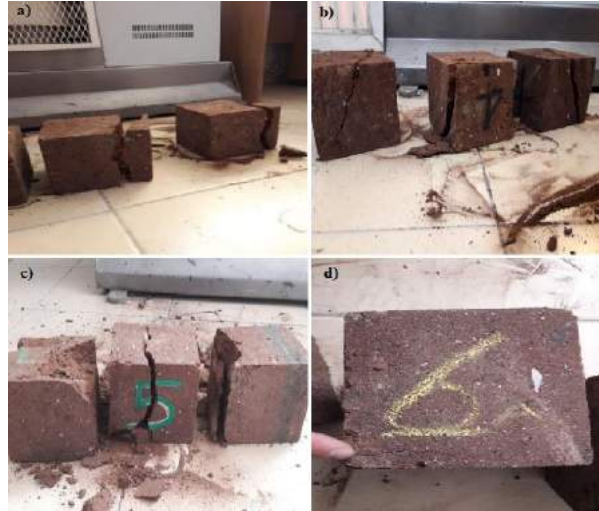
Fig. 6. Ahlat Stone Samples Broken after Drying Oven Curing
