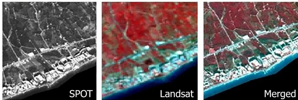
Figure 3: An example for spatial enhancement using PCA merging (left: SPOT panchromatic, center: Landsat TM, right: enhanced image)
