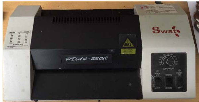
Figure 5. Laminating device used for the printed circuit.
