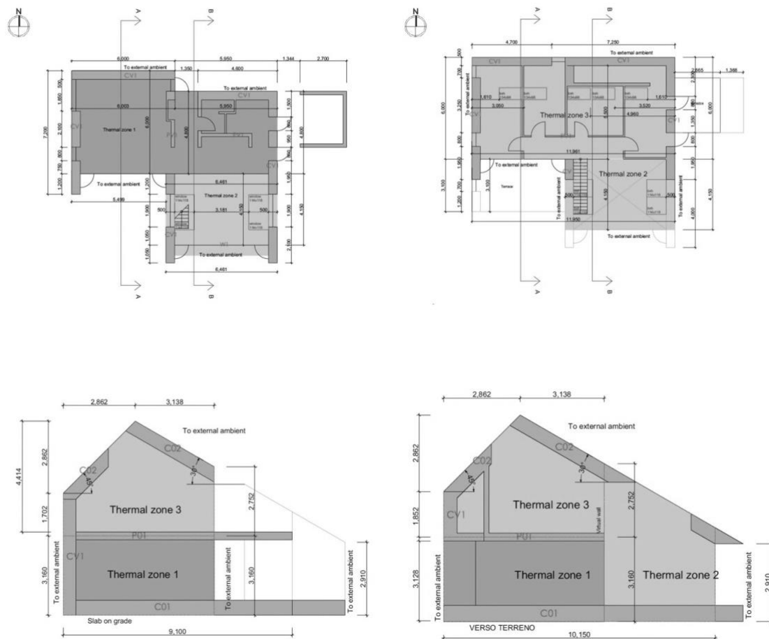
Fig. 1. Ground floor and section A-A on the left and second floor and section B-B on the right
