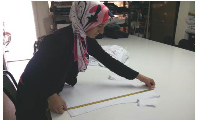
Figure 6. Operator's front length measurement
