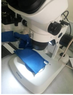
Figure 2. Image acquisition with Olympus digital microscope
