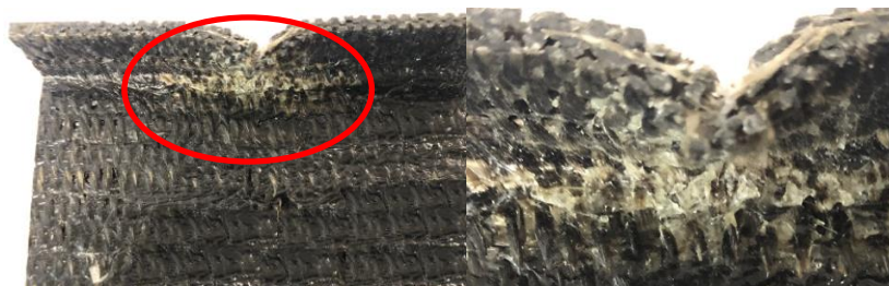
(c) The overall and partial enlargement failure modes on the web of the 3D I-shaped woven composite
