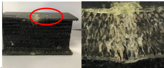
(a) The overall and partial enlargement failure modes on the top flange of the composites
