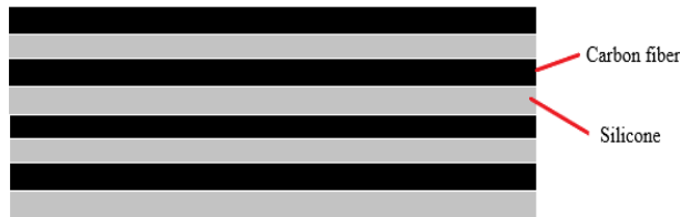
Figure 8. Representation of CFRS-C layered structure
