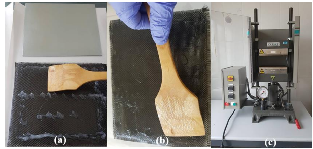
Figure 6. Manufacturing process of CFRS-C and the hot press machine utilised after hand lay up.
