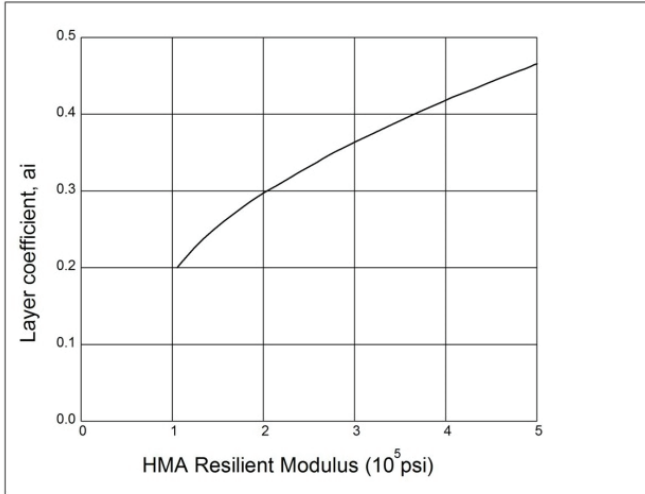
Figure 2 - Layer coefficients due to HMA resilient modulus [1]
