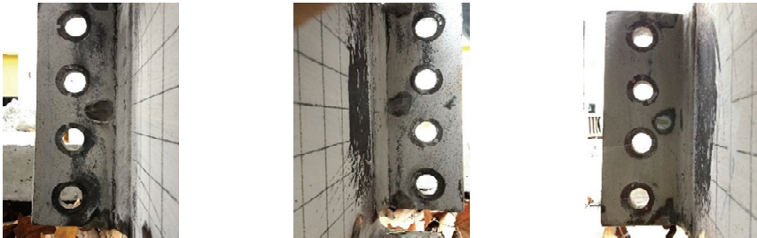
Figure 10 - End-plate deformations (left to right; T5-10, T5-15, T5-20)
